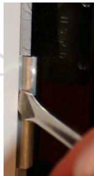
Carefully pry under magnets and twist slightly to adjust upwards.
